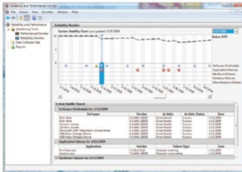
Figure 14-48 Use Reliability Monitor to search for when a problem began Courtesy: Course Technology/ Cengage Learning
