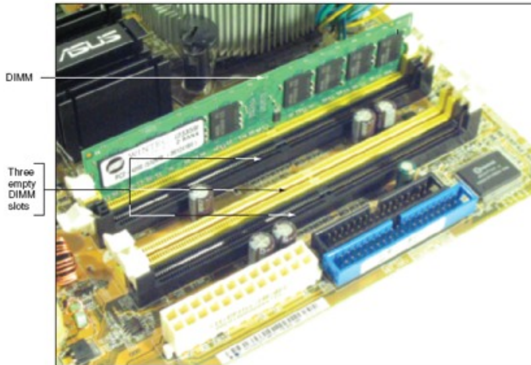
Figure 1-13 A DIMM holds RAM and is mounted directly on a motherboard
