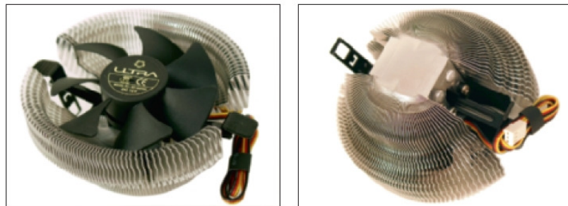
Figure 6-9 A cooler sits on top of a processor to help keep it cool Courtesy: Course Technology/Cengage Learning
