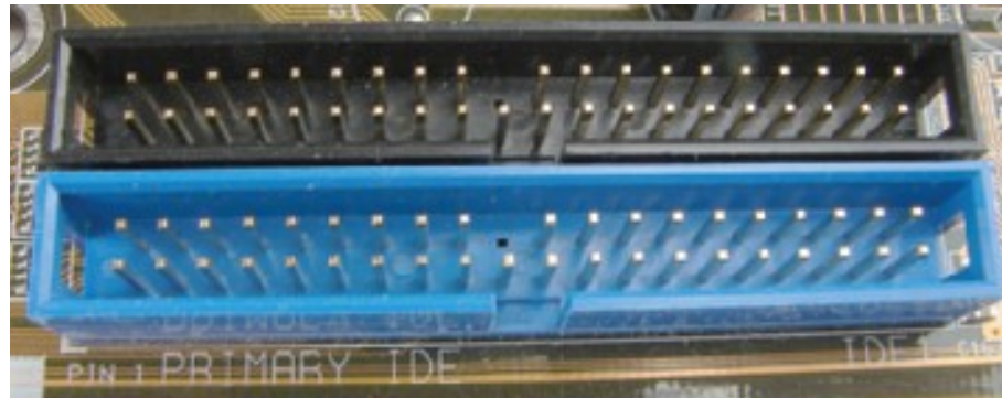
Figure 8-35 The primary IDE channel connector is often color-coded as blue Courtesy: Course Technology/Cengage Learning
