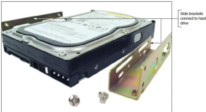
Figure 8-45 Use the universal bay kit to make the drive fit the bay
