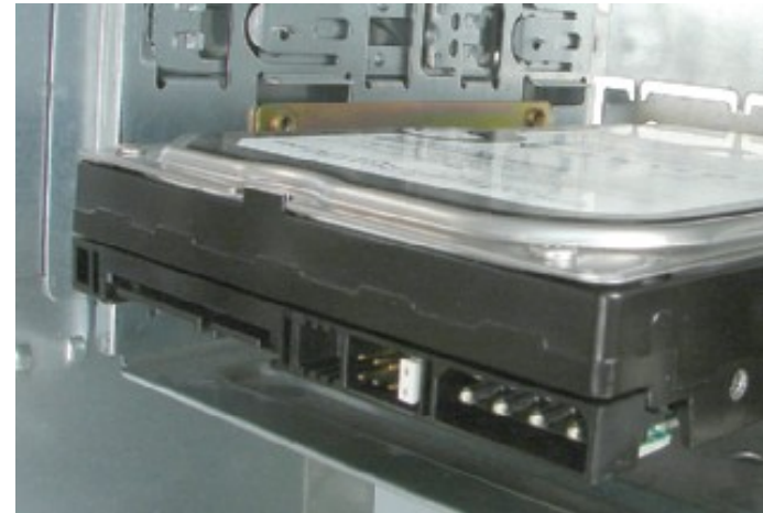
Figure 8-46 Hard drive installed in a wide bay using a universal bay kit adapter
