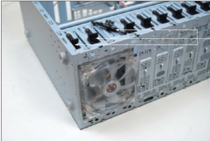
Figure 8-31 The removable bay has a fan in front and is anchored to the case with locking pins Courtesy: Course Technology/Cengage Learning
