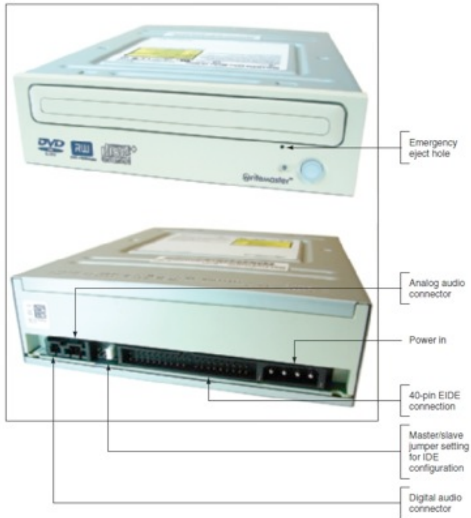
Figure 10-34 Front and rear of an EIDE DVD drive Courtesy: Course Technology/Cengage Learning
