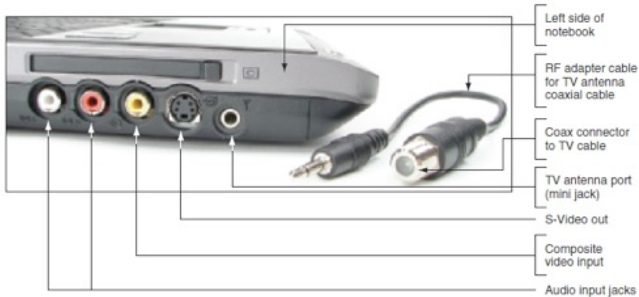
Figure 10-3 This notebook computer has embedded TV tuner and video capture abilities
