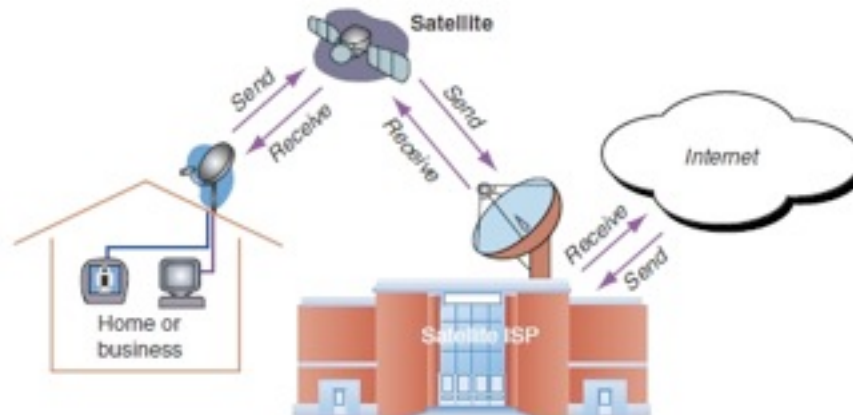
Figure 17-5 Communication by satellite can include television and Internet access Courtesy: Course Technology/Cengage Learning
