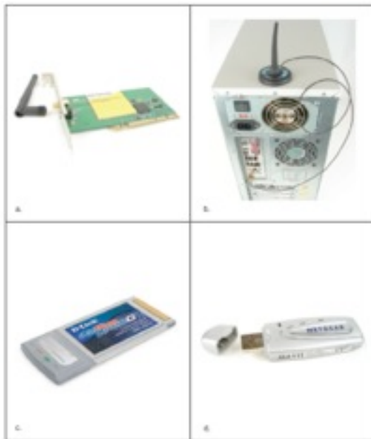
Figure 17-16 Four different types of wireless network adapters: (a) wireless NIC that fits in a PCI slot; (b) onboard wireless with an antenna that can be moved; (c) PC Card wireless NIC with embedded antenna; and (d) wireless NIC that uses a USB port on a desktop or notebook computer. Courtesy: Course Technology/ Cengage Learning
