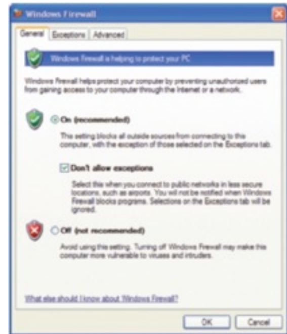
Figure 18-27 Windows Firewall for Windows XP is set for maximum protection. Courtesy: Course Technology/Cengage Learning
