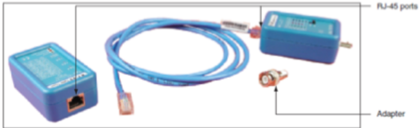
Figure 18-47 Use a cable tester pair to determine the type of cable and if the cable is good
