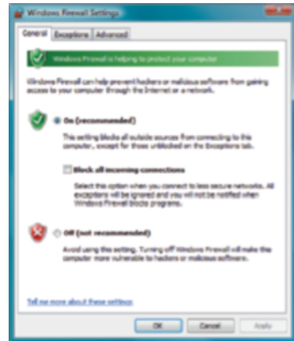
Figure 18-25 Windows Firewall is on but not working at its highest security level. Courtesy: Course Technology/Cengage Learning
