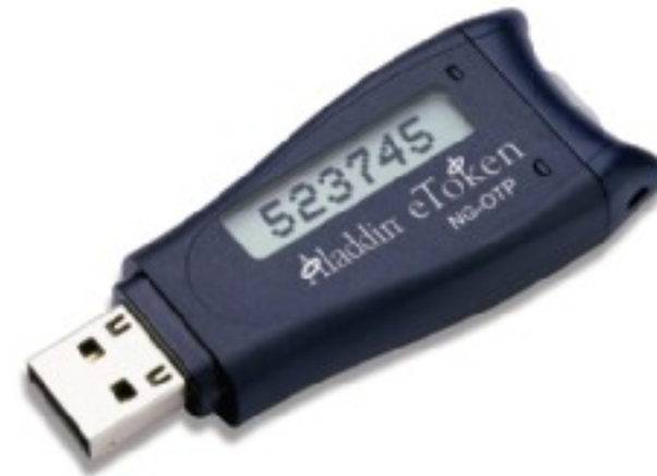
Figure 19-16 This eToken by Aladdin can contain digital certificates so that a user can do business over a VPN Courtesy of Aladdin
