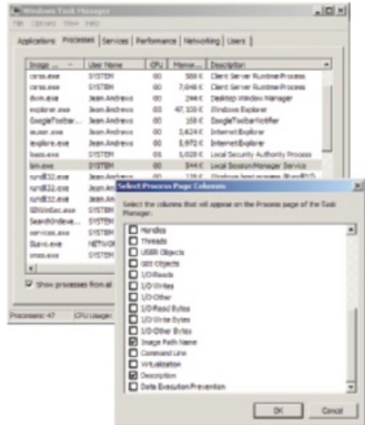
Figure 20-49 Set Task Manager to show the path to a program file Courtesy: Course Technology/Cengage Learning
