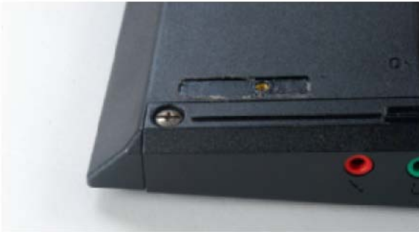
Figure 21-53 This one screw holds the hard drive in position Courtesy: Course Technology/Cengage Learning
