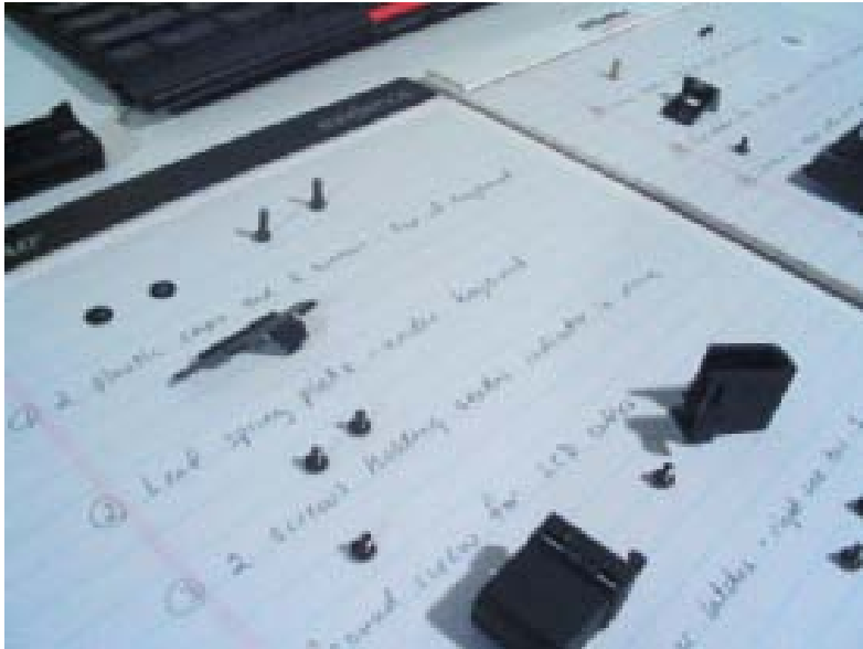
Figure 21-58 Using a notepad can help you organize screws so you know which screw goes where when reassembling Courtesy: Course Technology/Cengage Learning
