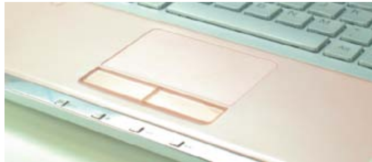
Figure 21-37 The touch pad is the most common pointing device on a notebook Courtesy: Course Technology/Cengage Learning
