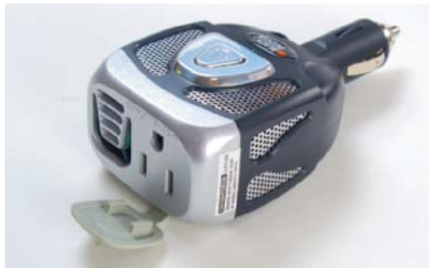
Figure 21-25 An inverter changes DC to AC and provides an outlet for your laptop's AC adapter Courtesy: Course Technology/Cengage Learning
